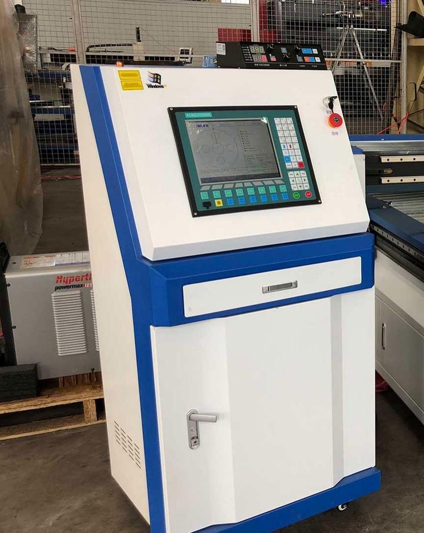
Plasma Controller For Gantry Type CNC Cutting Machine, Supports Computer Control Windows XP/2000
